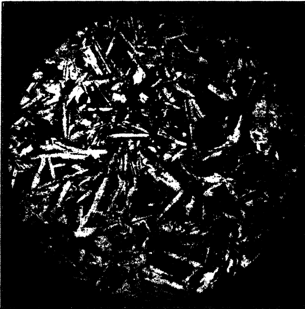
FIG. 47.—Photomicrograph of a section of Diabase. (Photo. loaned by A. B. Cushman.)
